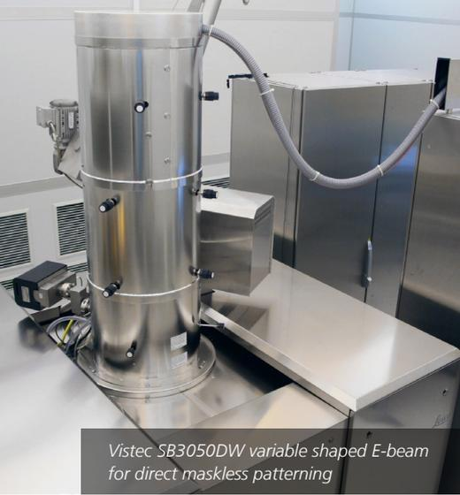
Vistec SB3050DW variable shaped E-beam for direct maskless patterning
