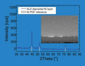
2 left: XRD phase analysis of Ni thin film deposited by PE-ALD, showing an fcc-nickel phase. Inset: SEM tilted view image of the same layer.
