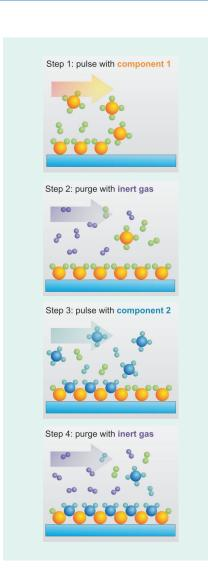
3 ALD Mechanism: The ALD cycle of a metal oxide deposition is composed of the following steps: metal-containing precursor pulse (step 1), purge of non-reacted precursor and reaction products with inert gas (step 2), oxidant pulse e.g. ozone or water (step 3) and a second inert gas purge to remove reaction products (step 4). The sequence is repeated several times to achieve the desired film thickness
