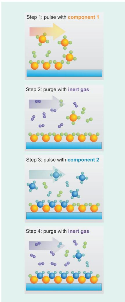
3 ALD Mechanism: The ALD cycle of a metal oxide deposition is composed of the following steps: metal-containing precursor pulse (step 1), purge of non-reacted precursor and reaction products with inert gas (step 2), oxidant pulse e.g. ozone or water (step 3) and a second inert gas purge to remove reaction products (step 4). The sequence is repeated several times to achieve the desired film thickness.
