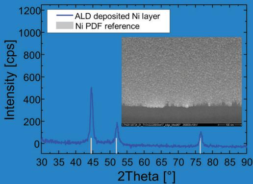
2 left: XRD phase analysis of Ni thin film deposited by PE-ALD, showing an fcc-nickel phase. Inset: SEM tilted view image of the same layer.
