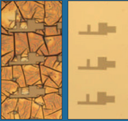
▲ Nanostructured sample before (left) and after photo resist removal (right).
